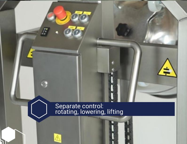
Separate control: rotating, lowering, lifting
