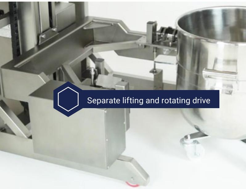
Separate lifting and rotating drive
