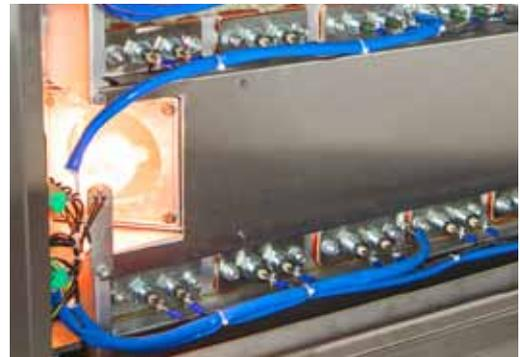
No control components such as contactors, fuses or relays are installed on the oven walls. To protect them against adverse effects of high temperature, they were moved to one stainless electric box. This additionally facilitates supervision and maintenance of the oven.
