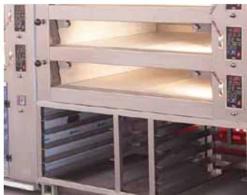
Loaders guarantee quick oven loading and unloading operations.
