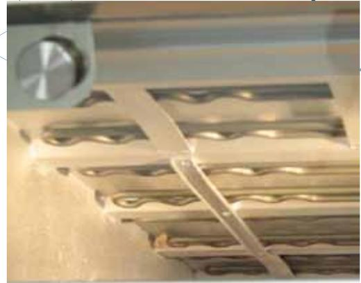
Each heater is fixed separately, which prevents it from sliding out during operation (heating/cooling).
