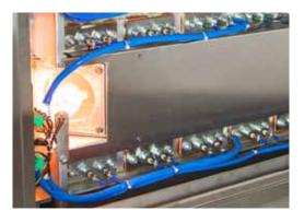
No control components sucgh as contactors, fuses or relays are installed on the oven walls. To protect them against adverse effects of high temperature, they were moved to one stainless electric box. This additionally facilitates supervision and maintenance of the oven.
